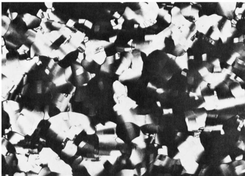
FIGURE 2 Optical texture observed with: 2a: HAB C_7 derivative at 81^\circ\text{C} 2b: HET C_5 derivative at 82^\circ\text{C}
