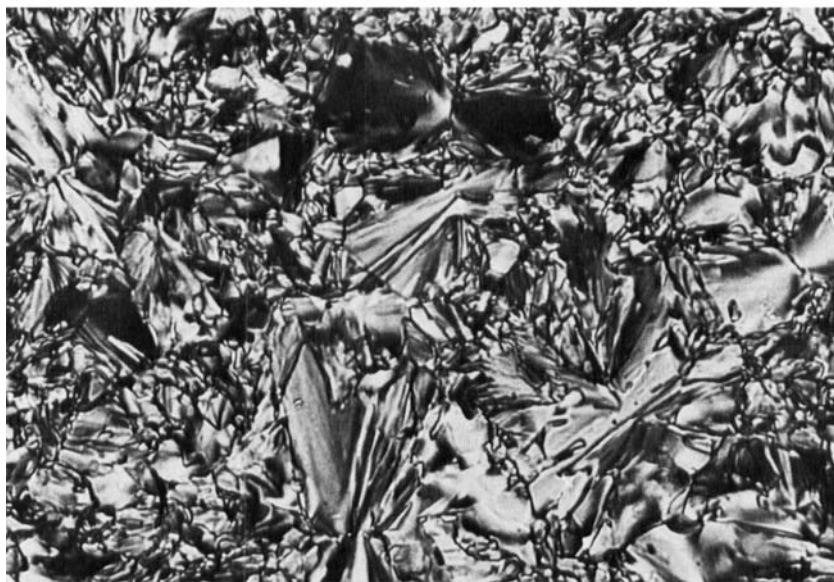
FIGURE 4 Optical texture observed with the C_8O HBT derivative: 4a: N_D nematic phase at 200^\circ C 4b: Columnar phase at 160^\circ C
